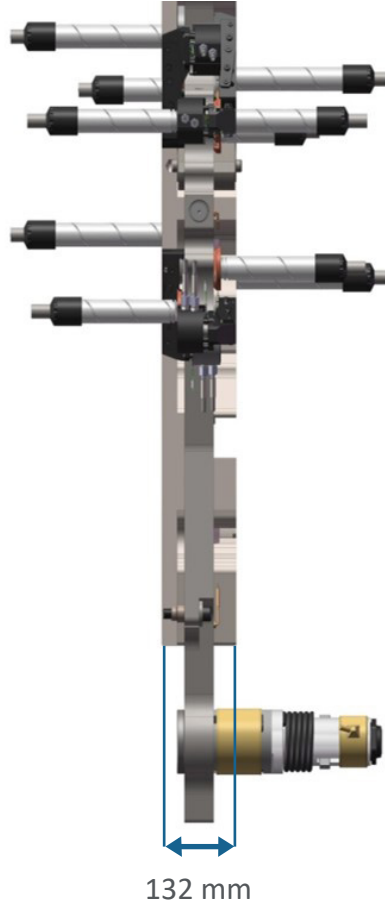
SHIFTED NOZZLES One manifold version
